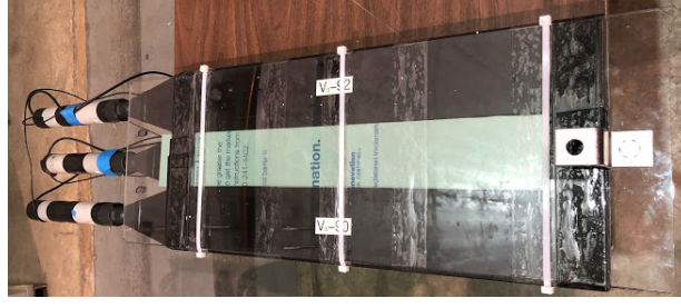
Figure 3.30: Photograph of S3 scintillator used in CREX. It is a combination of three PREX-2 style S3 scintillators. Signals from the three PMTs are combined using logical OR so that the combination works as a single body.
