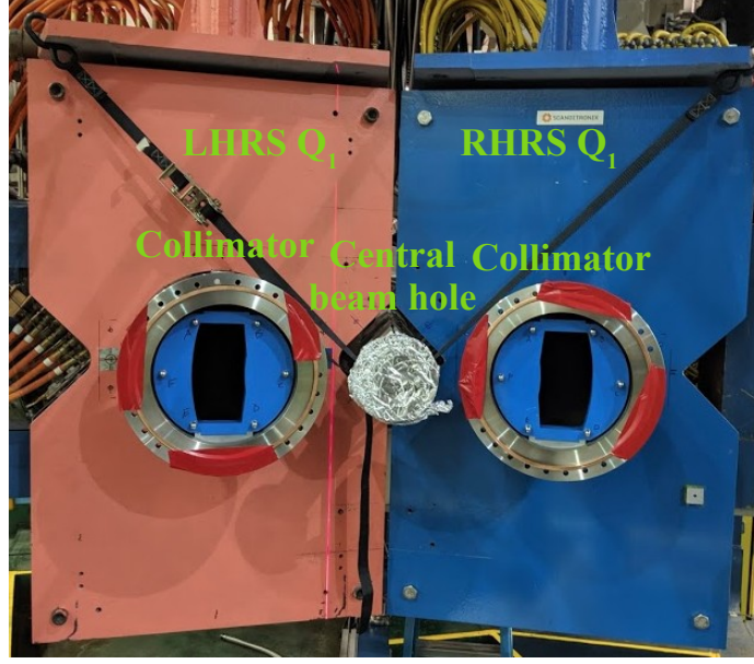
Figure 3.23: Photograph during installation of the PREX-2/CREX acceptance-defining collimators for the left and right HRSs. The left and right collimators are symmetric with respect to the beamline which is shown in between the two collimators.
